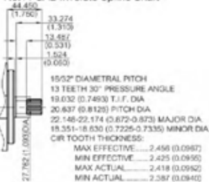
25HM Series No.11 SAE Involute Spline Shaft
